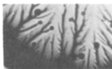
Fig. 7 Solidification of the eutectic mixture of the nitrates
